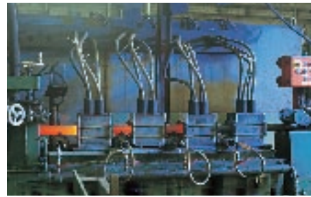
Induktive Einzelstabvergütung Induction hardening and tempering of single bars
